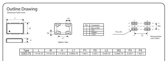
$Quartz\ crystal\ oscillators\ house\ a\ small\ 5x7mm\ package.\ Choice\ of\ 3.3V\ and\ 5V\ supply\ versions.$
